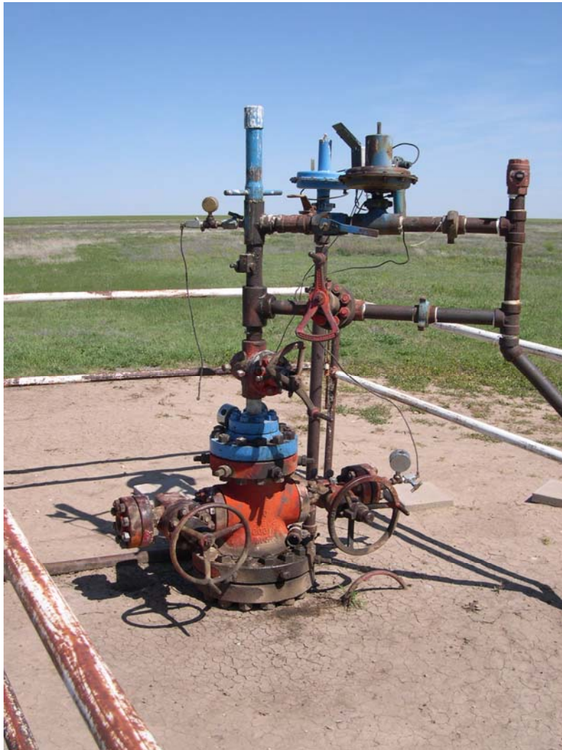
Figure 3 - Typical Flange Wellhead with Tubing Plunger Installation Prior to Modification for Casing Plunger Application
