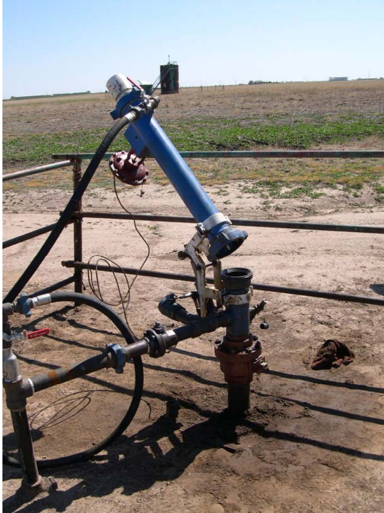
Figure 8 - Fully Assembled Casing Plunger Lubricator Power assisted lift (Pat. Pend.) is helpful on 4 ½ inch casing plungers and essential on 5 ½ inch casing plungers.
