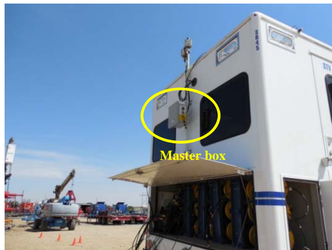
Figure 5 - TMV3H45 and master box of the level monitoring system
