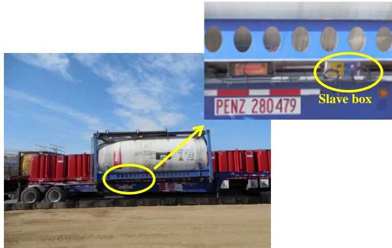
Figure 4 - The isotainer tank used to test proposed level monitoring system
