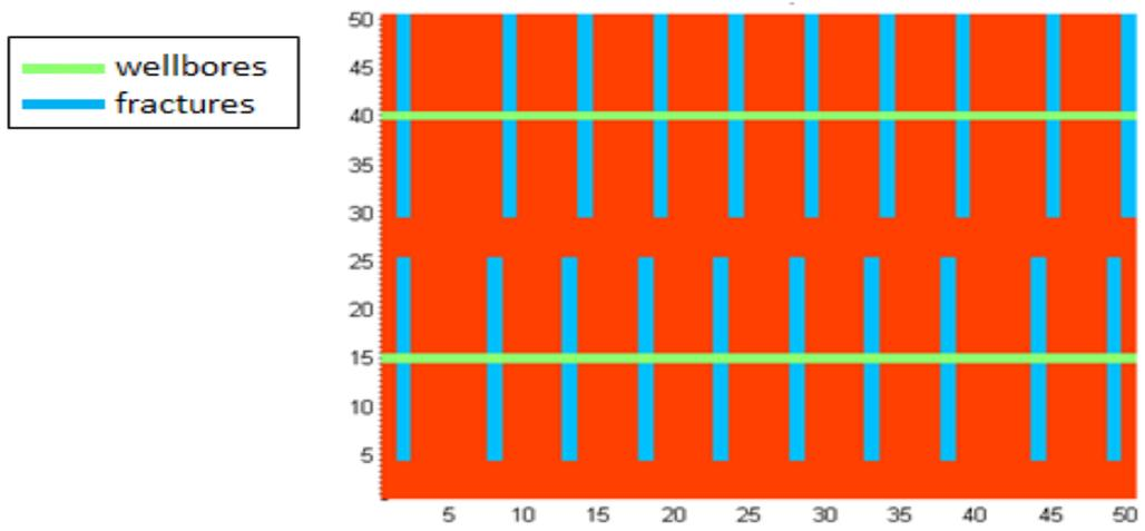
Figure 27: Optimal Placement for a Maximum Fracture Half-length of 10 and No Overlap
