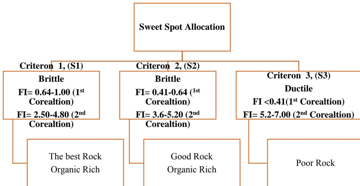
Figure 7: The developed sweet spot selection methodology for placing wells and fractures in shale reservoirs (this paper)
