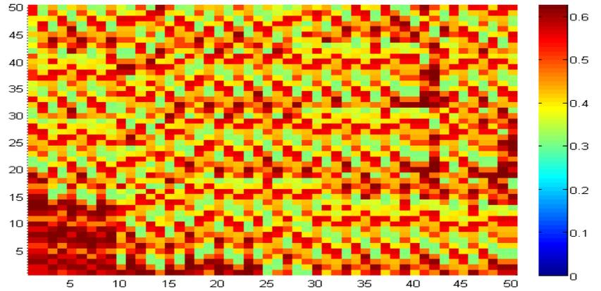
Figure 26: Fracturability Index map based on the tested shale model
