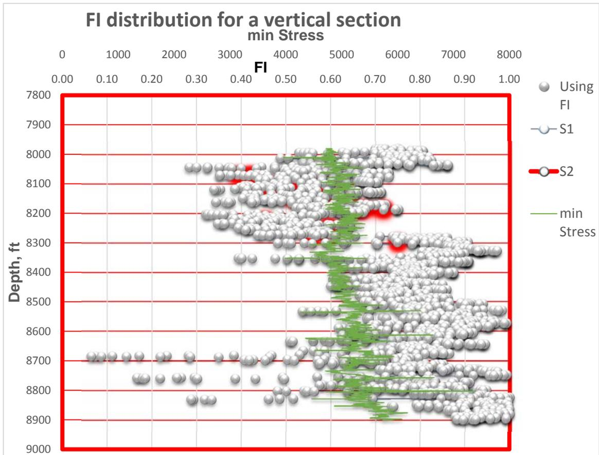
Figure 20: New developed FI screened by S1, S2 and min stress profile versus depth
