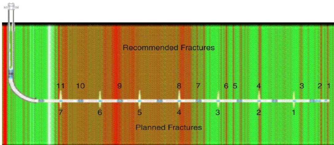
Figure 2- The brittleness track shows variation in rock heterogeneity, the red section is more brittle after parker et al. (2009)
