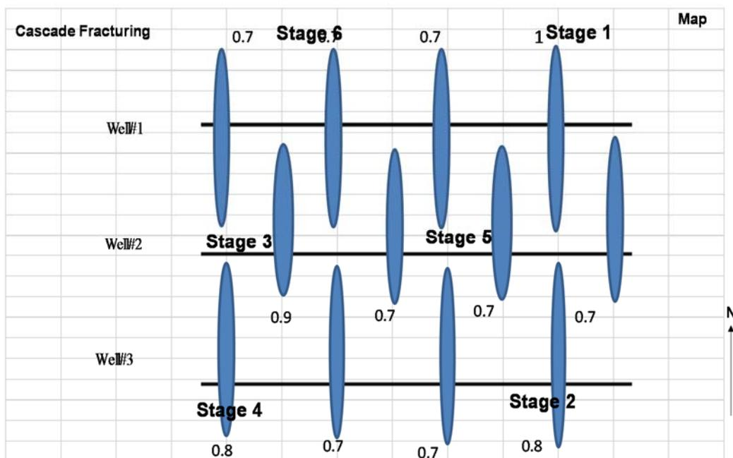
Figure 24: Schematic of a map view of suggested fracture stages suggested by FI values.
