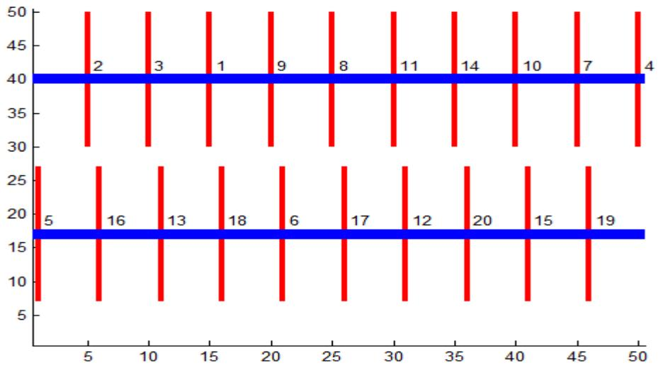
Figure 28: Sequencing of fractures according to FI values.
