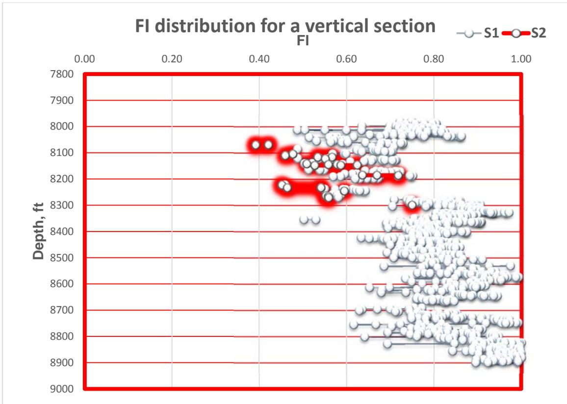
Figure 19: New developed FI screened by S1 and S2 conditions versus depth
