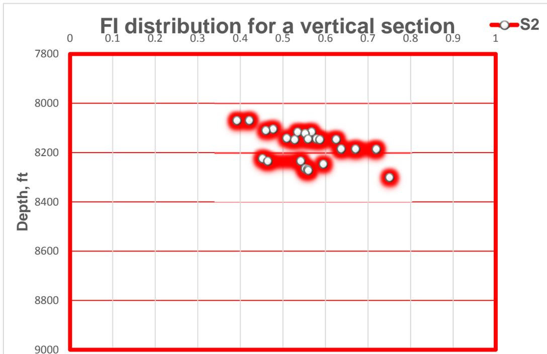
Figure 18: New developed FI screened by S1 conditions versus depth
