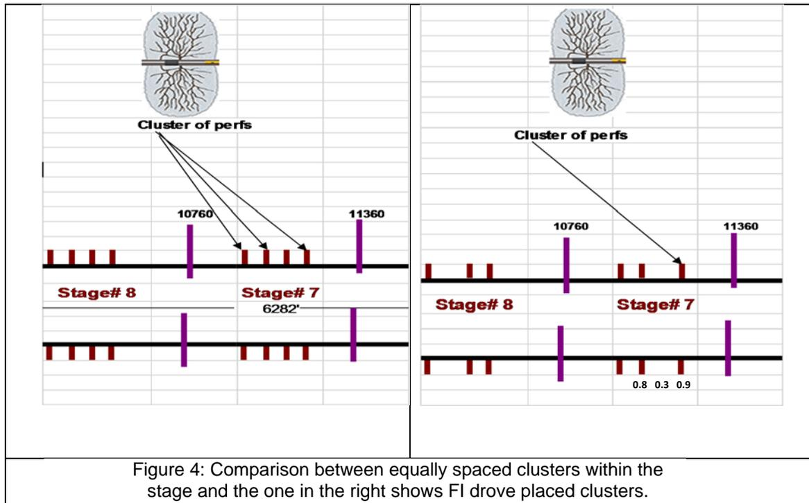
Figure 4: Comparison between equally spaced clusters within the stage and the one in the right shows FI drove placed clusters.
