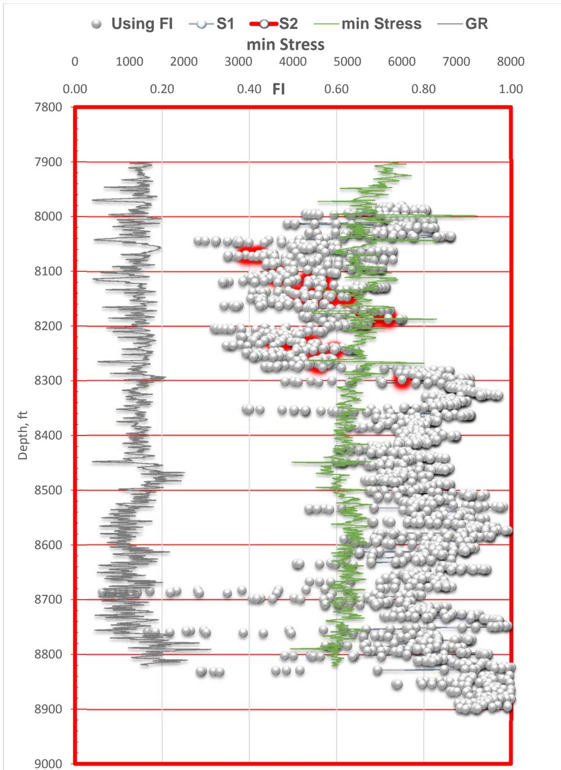
Figure 21: New developed FI screened by S1, S2 , min stress and gamma ray profile versus depth
