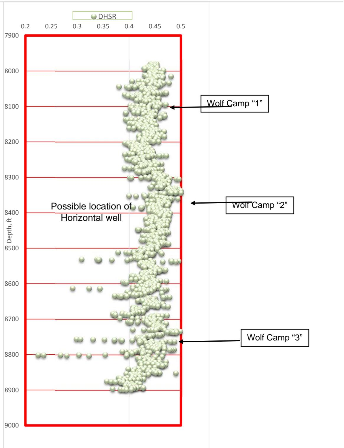
Figure 11: Differential Horizontal stress ratio versus depth.
