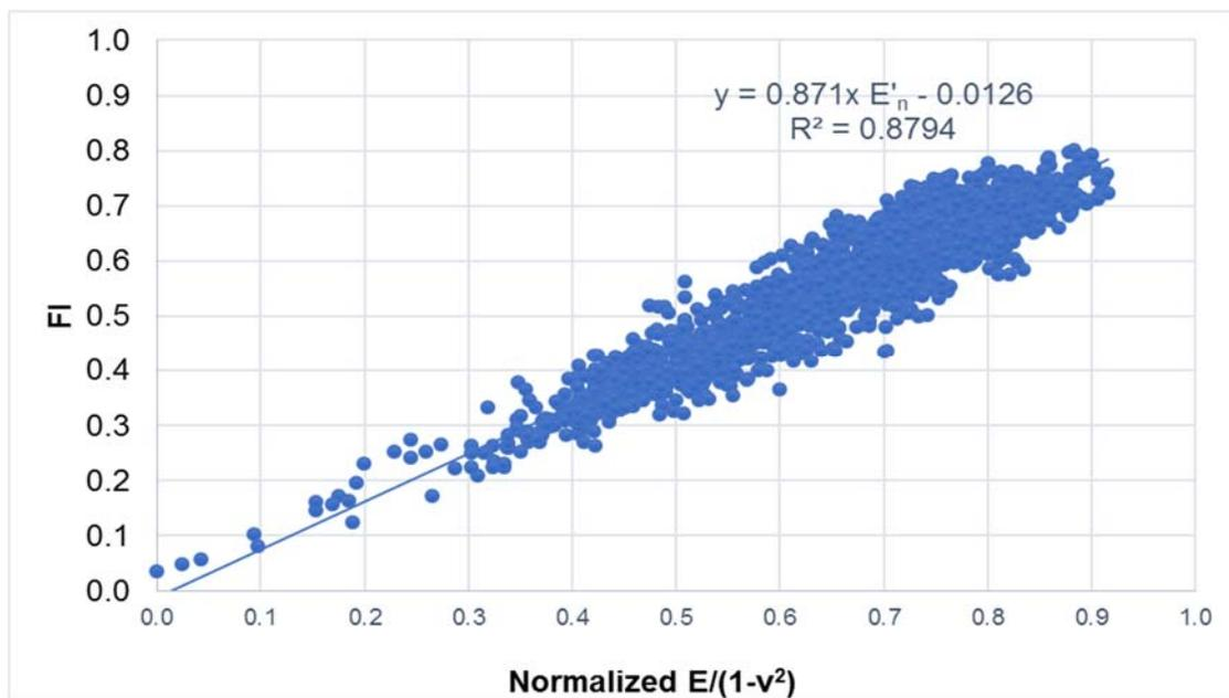
Figure 8: A geomechanical based FI correlation introduced by Alzahabi et al. 2015
