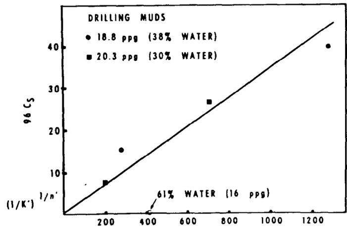
FIGURE 10—DEPENDENCE OF THE SLIP COEFFICIENT UPON CONSISTENCY INDEX ( $K'$ ) FOR HIGH DENSITY DRILLING MUDS.
