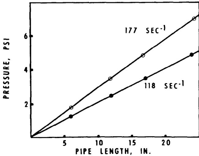
FIGURE 5—PRESSURE DROP AS A FUNCTION OF PIPE LENGTH, DEMONSTRATING THE VALIDITY OF EQ 15 (LONGHORN H, 40% WATER, 0.57% HEC, 80°F).
