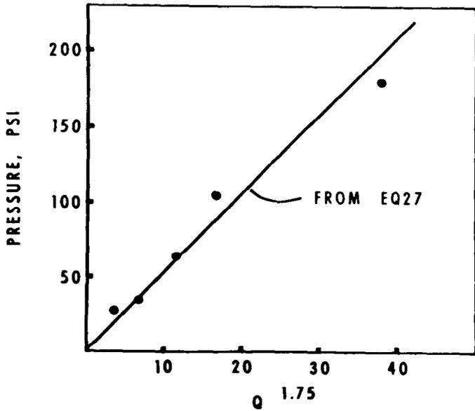
FIGURE 12—TURBULENT FLOW BEHAVIOR OF WATER FLOWING THROUGH A 1.815" I.D. PIPE. THE LINE WAS CALCULATED USING EQ 27.
