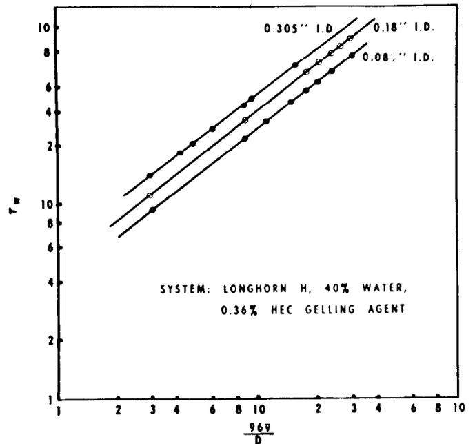
FIGURE 4—GRAPHICAL LOG-LOG PLOT EXEMPLIFYING THE POWER LAW BEHAVIOR OF PIPE-FLOW RHEOLOGICAL DATA.
