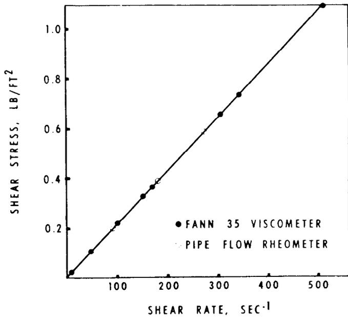
FIGURE 2—SHEAR STRESS-SHEAR RATE RELATIONSHIP OF A 103 CP NEWTONIAN OIL.
