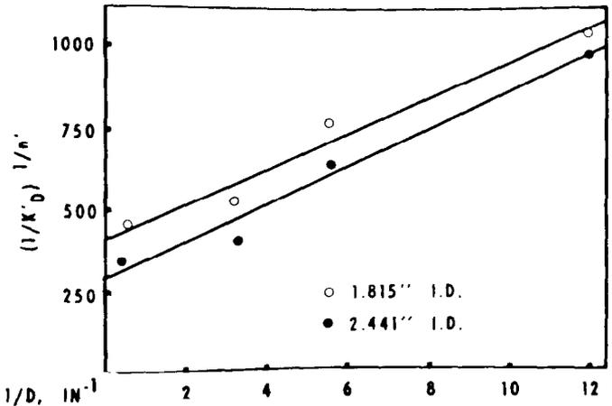
FIGURE 15—SCALE UP OF RHEOLOGICAL MEASUREMENTS (USING PIPEFLOW RHEOMETER) OF TWO SEPARATE MIXES OF OKLAHOMA CLASS H CEMENT SLURRIES (38% WATER, 0.1% RETARDER, 0.1% PREHYDRATED BENTONITE, 98°F.)
