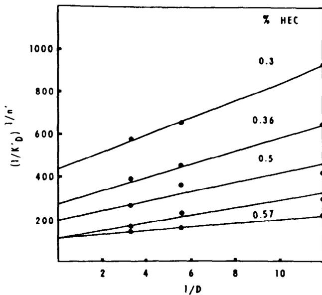
FIGURE 7—DEPENDENCE OF THE CONSISTENCY INDEX,  $K'D$  UPON PIPE DIAMETER (OKLAHOMA CLASS H, 40% WATER, 80°F).
