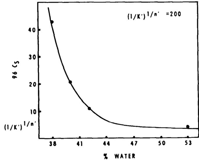
FIGURE 9—DEPENDENCE OF THE SLIP COEFFICIENT UPON CEMENT WATER CONTENT.
