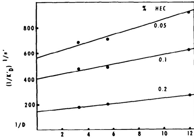
FIGURE 6—DEPENDENCE OF THE CONSISTENCY INDEX,  $K'D$  UPON PIPE DIAMETER (OKLAHOMA CLASS H, 42% WATER 80°F).
