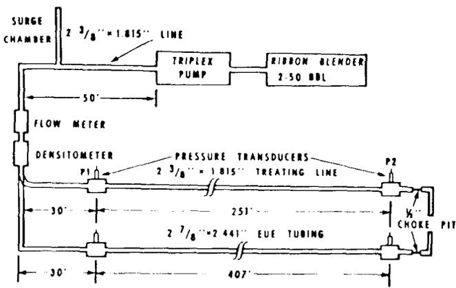
FIGURE 11—SCHEMATIC DIAGRAM OF RHEOLOGICAL TESTING AT DOWELL TRAINING CENTER KELLYVILLE, OKLAHOMA.
