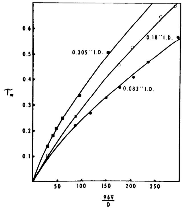
FIGURE 3—RHEOLOGICAL MEASUREMENTS USING THE PIPE-FLOW RHEOMETER DEPICTED IN FIGURE 1 (LONGHORN H, 40% WATER, 0.36% HEC, 80°F).
