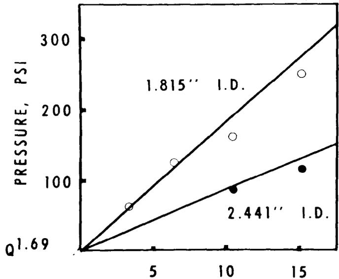
FIGURE 16—TURBULENT FLOW BEHAVIOR OF THE CEMENT SLURRY FLOWING THROUGH PIPE. THE LINES WERE CALCULATED USING EQ 30 AND 31.
