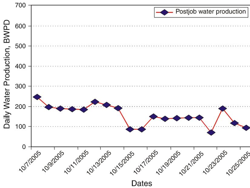
Figure 13b — Water production rate of the well *after* treatment with water conformance polymer and consolidating treatment fluids.
