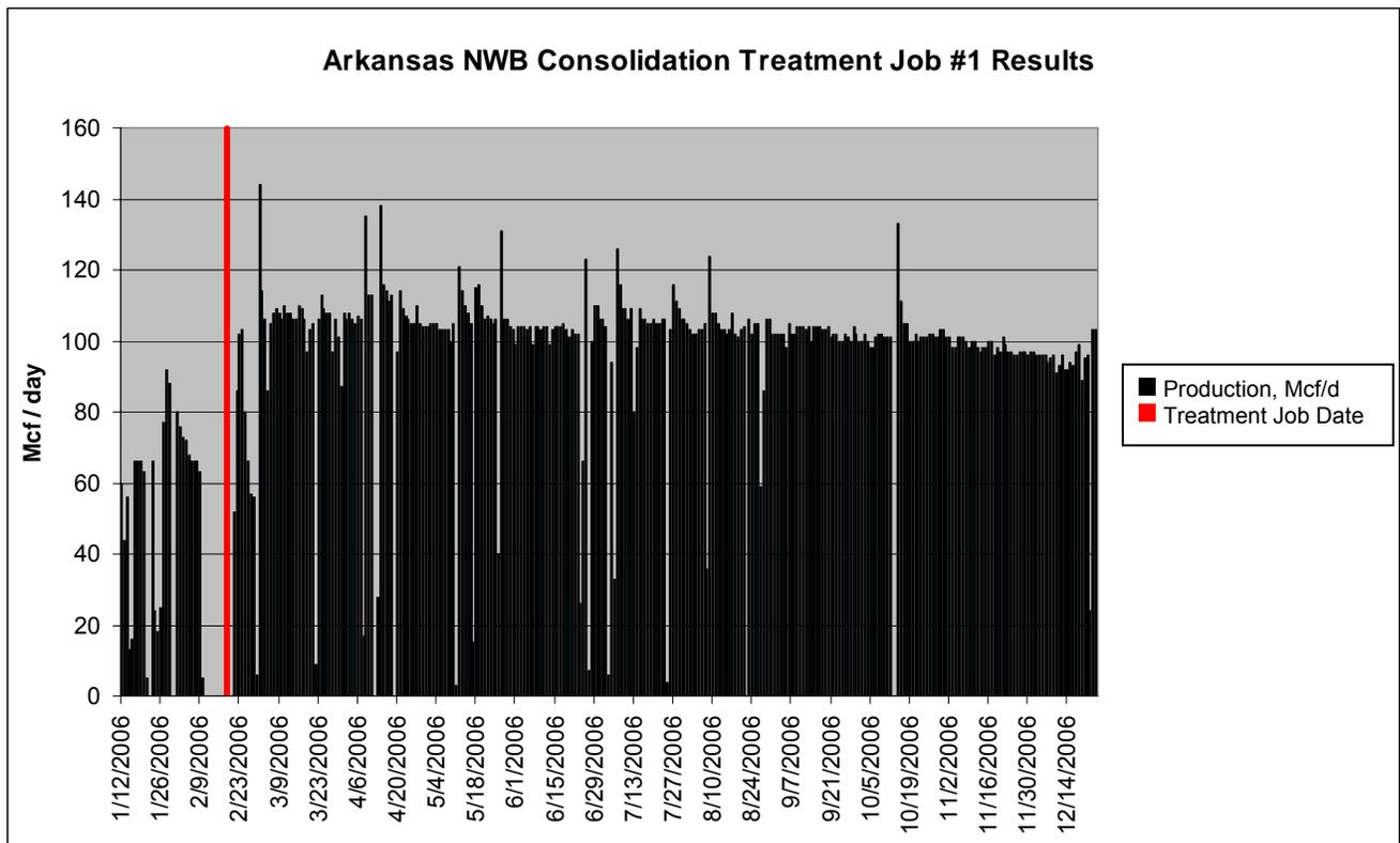
Figure 12a — Production results from Arkansas Well 1. In 10 months, one trip was made to the wellhead post-treatment to check for sand fill; none was found. This well has pumped continually for 10 months with no interruption.
