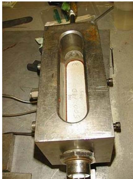
Figure 3—Interior view of a modified API linear conductivity cell.
