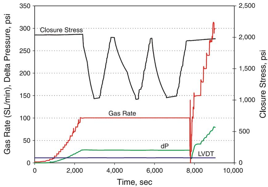
Figure 5—Flow of heated gas to simulate gas production through sand pack treated with liquid curable resin at 175°F.
