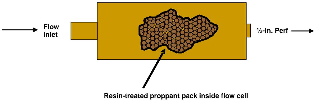
Figure 2a — Schematic diagram showing the proppant pack and flow directions through the flow cell. The flow cell was used in packing proppant, applying consolidation treatment, and testing flowback with water.
