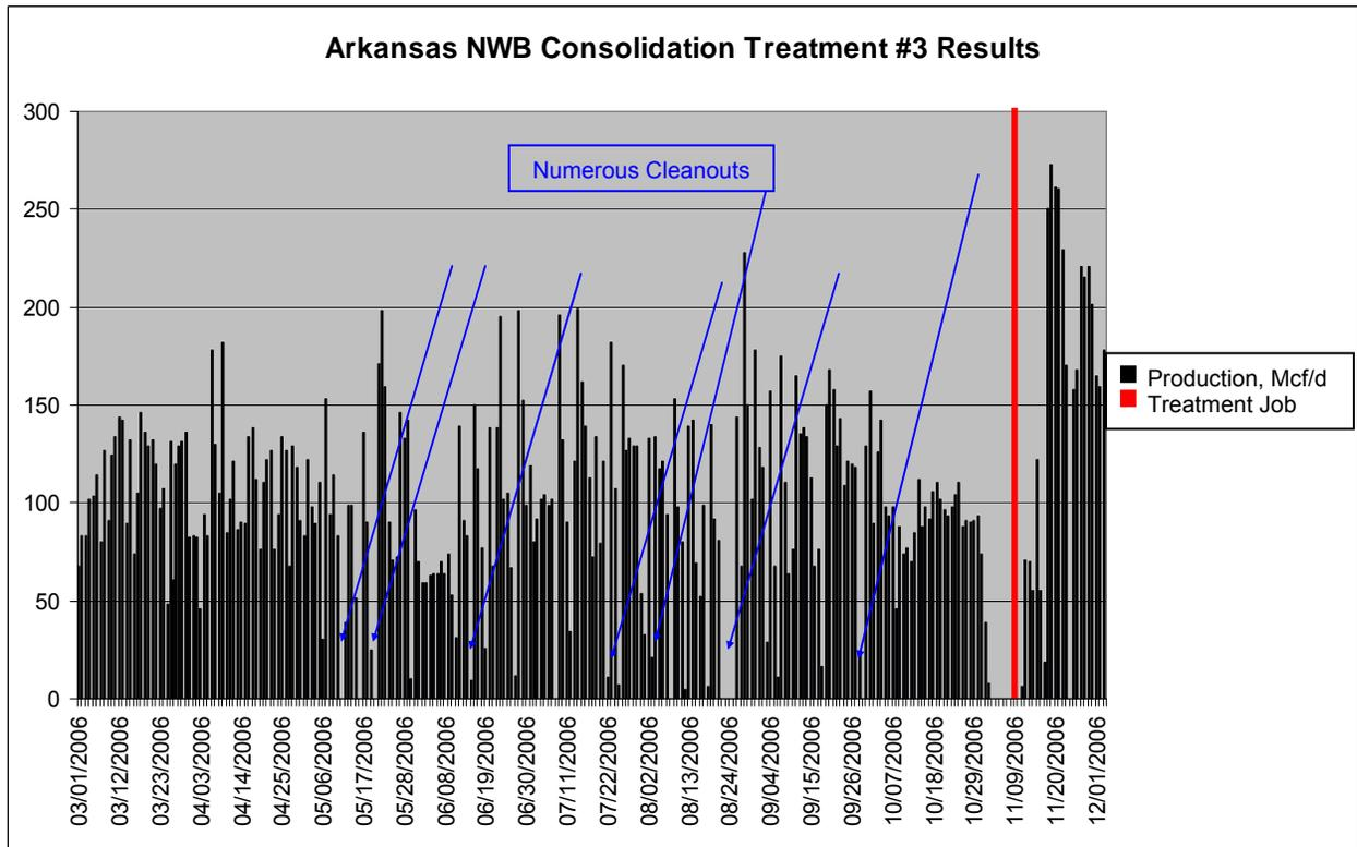
Figure 12c — Production results from Arkansas Well 3. Substantial initial production increase has been witnessed due to efficiently sustaining the rod pump system. The blue arrows highlight the extensive wellbore clean out history prior to the consolidation treatment shown in red.
