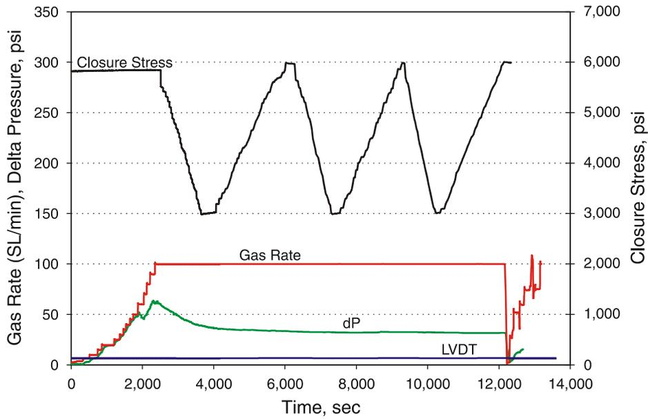
Figure 9 — Flow of heated gas to simulate gas production through bauxite proppant pack that has been treated with liquid curable resin at 350°F.
