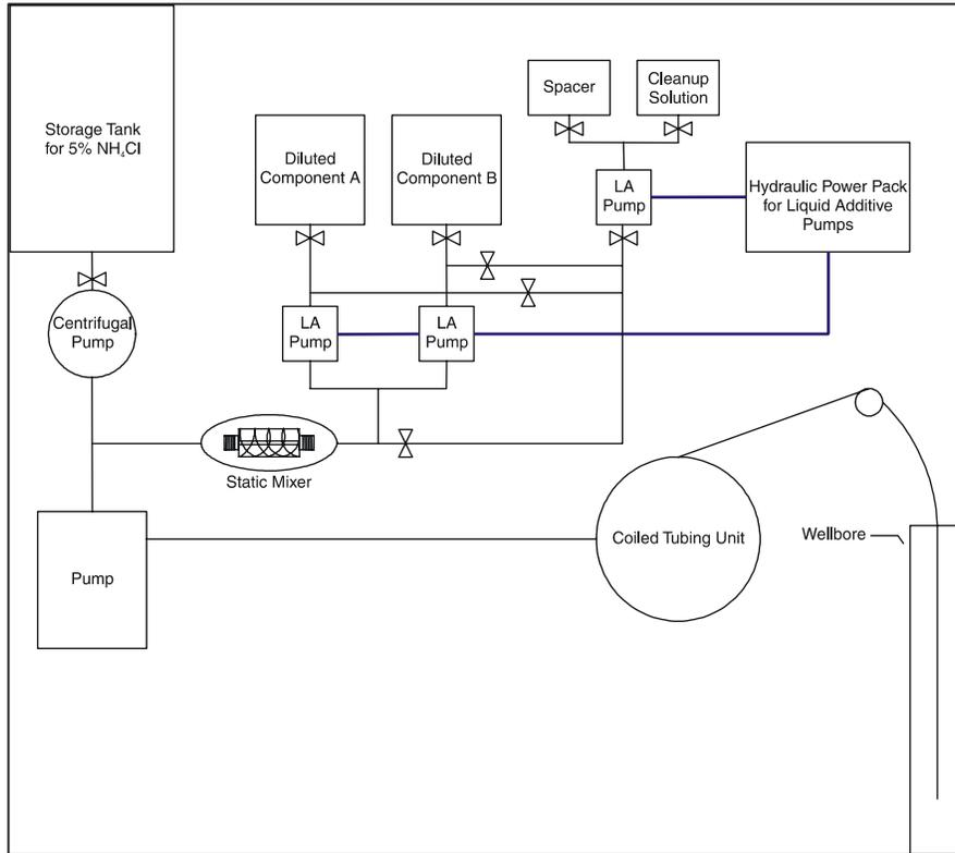
Figure 11—Schematic layout of equipment involved at wellsite for remedial proppant treatment.
