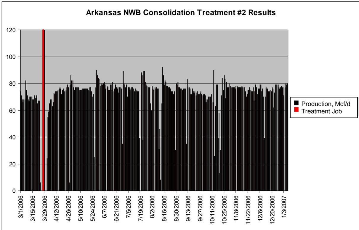
Figure 12b — Production results from Arkansas Well 2. In 9 full months since the treatment, no maintenance work has occurred on this well.
