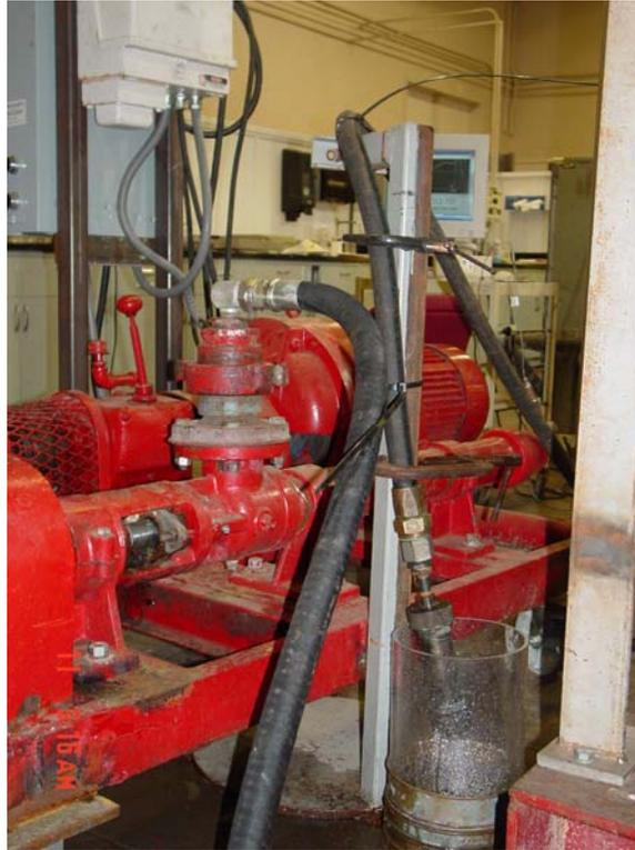
Figure 2b — A progressive cavity pump was used in pumping water through the proppant pack at various flow rates to determine the resin performance in controlling flowback of the proppant.
