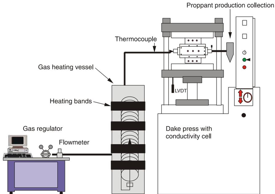
Figure 4 — Schematic diagram of equipment involved in lab flowback testing using high-temperature, high gas flow rates.
