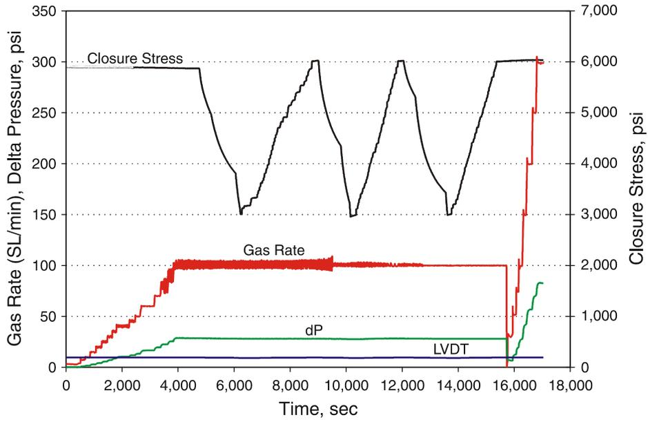
Figure 8 — Flow of heated gas to simulate gas production through bauxite proppant pack that has been treated with liquid curable resin at 250°F.
