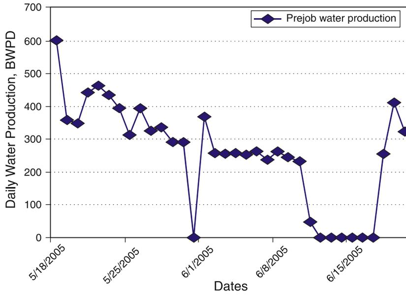
Figure 13a — Water production rate of the well *before* treatment with water conformance polymer and consolidating treatment fluids.
