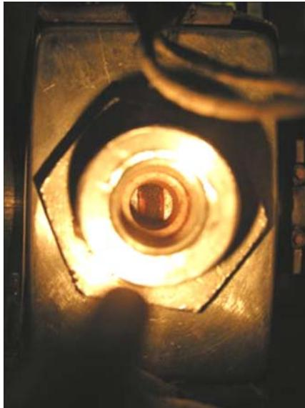
Figure 6—Close-up view of the proppant pack at the outlet end of the flow cell.
