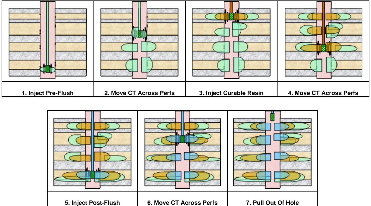
Figure 10 — Treatment process uses a combination of CT, resin consolidation, and pulsing tool Technologies to provide remedial solutions to help control proppant flowback.
