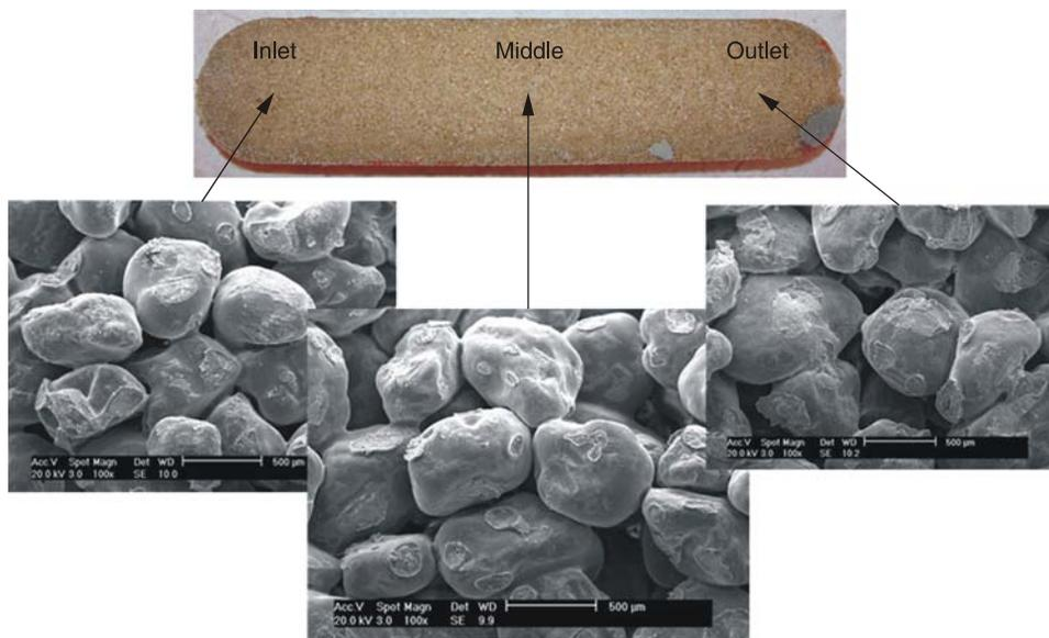
Figure 7 — SEM micrographs of sand pack taken at various locations showing the footprints of contact points and pore spaces between sand grains.
