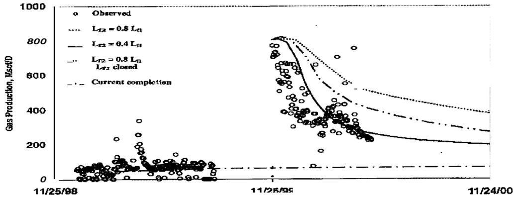
Figure 8 - Production History Match on Well A in Barnett Shale for Parallel and Orthogonal Refractures ( $L_{11}$  is initial fracture length,  $L_{12}$  is refracture length)
