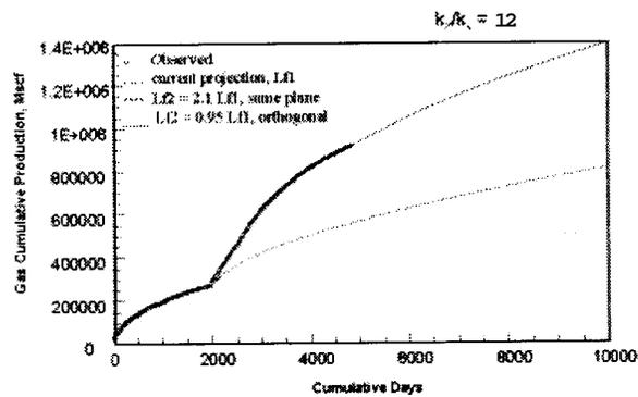
Figure 3 - Production history match on refractured Well C in Barnett shale for parallel and orthogonal refractures ( $L_{11}$  is initial fracture length,  $L_{12}$  is refracture length)
