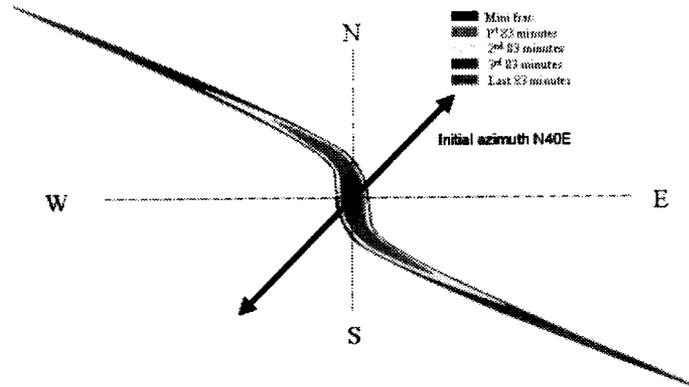
Figure 7 - Plan View of Well A Refracture Azimuth Growth as a Function of Time
