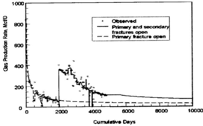
Figure 2a - Production History of Well C Before and After Successful Refracture Treatment
