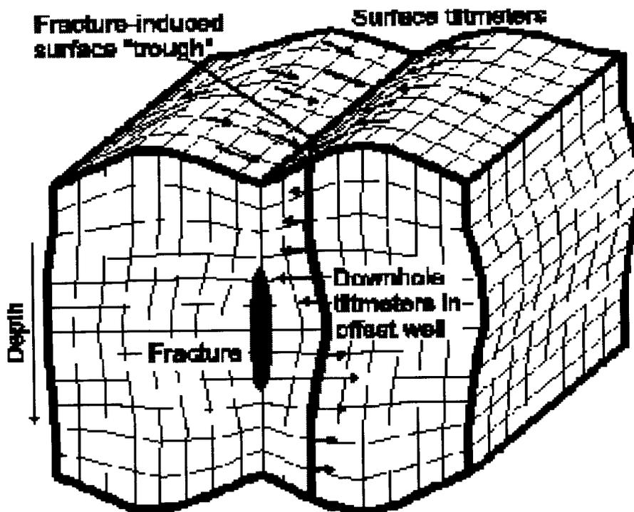
Figure 13 - Displacement Field in the Earth Around a Vertically Oriented Hydraulic Fracture, Showing Induced Surface and Downhole Tilt Vector Directions
