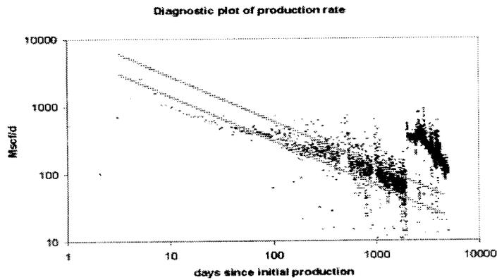
Figure 2b - Log-Log Plot of Production History of Well C Before and After Successful Refracture Treatment
