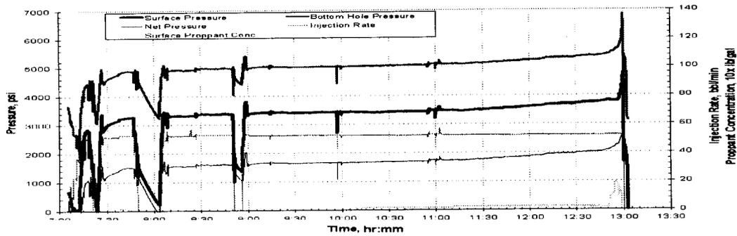
Figure 9 - Treatment Schedule for Well B Refracture Job
