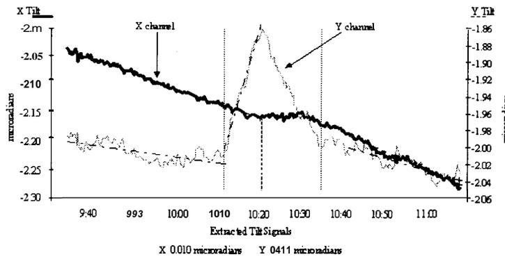
Figure 6- Raw Tiltmeter Signal for Main Frac Treatment on a Lost Hills, CA, Site Showing Abrupt Azimuth Change at Time 10:20
