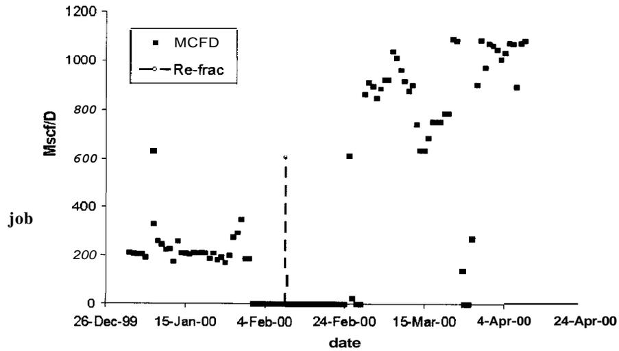
Figure 10 - Gas Production Versus Time, Before and After Refracture Treatment. From Well B
