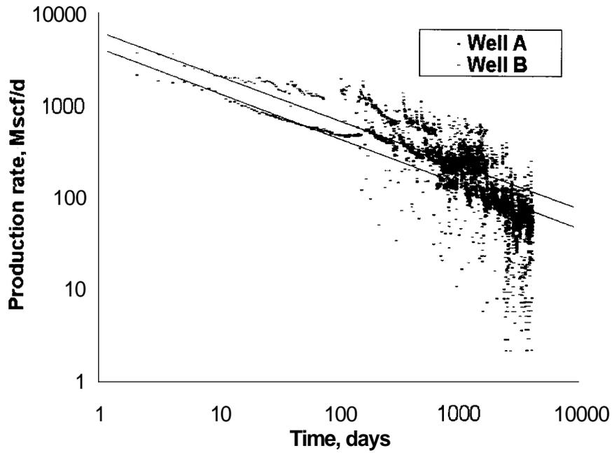
Figure 11- Log-Log Plot of Production History of Well A and Well B Before Refracture Treatment
