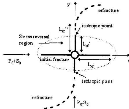
Figure 1 - Refracture Reorientation Concept
