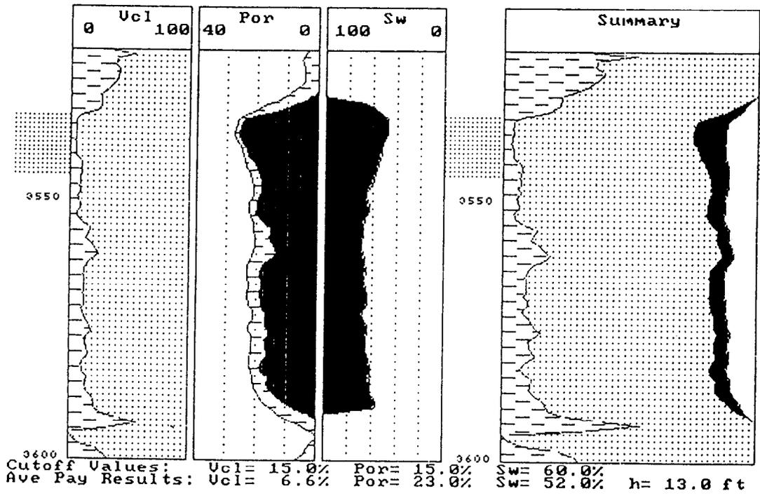
Figure 11b - Net Pay Summary for the potentially productive Bell Canyon sand 1077 to 1094 meters (3532 to 3590 feet). Note that there is 4 meters (13 feet) of net pay indicates with a concomitant hydrocarbon pore-meter thickness of 0.43 (1.4 pore-feet) using the following net pay cutoffs:
