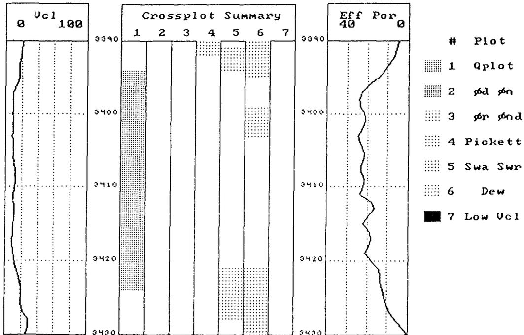
Figure 12b - Crossplot Summary for the potentially productive Cherry Canyon sand 1035 to 1044 meters (3396 feet to 3424 feet). Note that in columns 3 - 5 (hydrocarbon versus water crossplots) the zone appears productive over the permeable interval shown in column 1.
