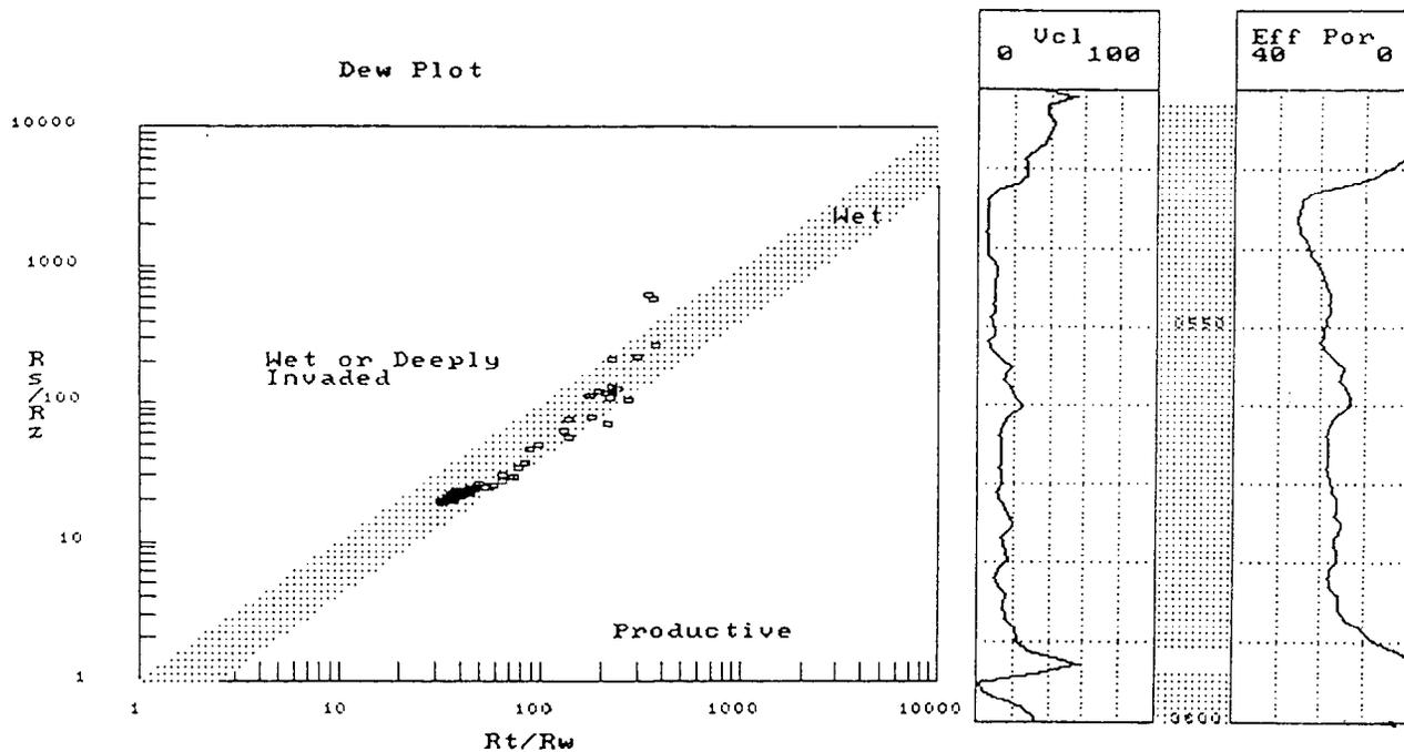
Figure 9 - Dew Plot ( $R_s/R_z$  versus  $R_t/R_w$ ) for the Bell Canyon sand. Note that all of the data cluster above the productive line ( $Sw/S_{xo} > 0.7$ ) indicating a lack of moved hydrocarbons. This lack of moved hydrocarbons is the result of the low permeability (i.e. high residual hydrocarbons see: Figure 5).
