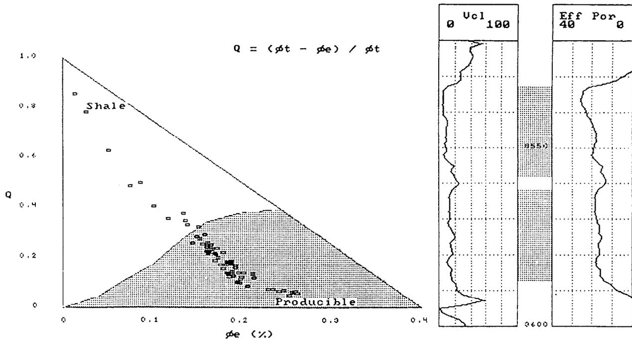
Figure 4 - Shaly Sand Producibility Plot (q-Plot) with volume of clay (Vcl) calculated from the gamma ray log for the Bell Canyon sand. Note that the majority of the data cluster in the producible region of the plot.
