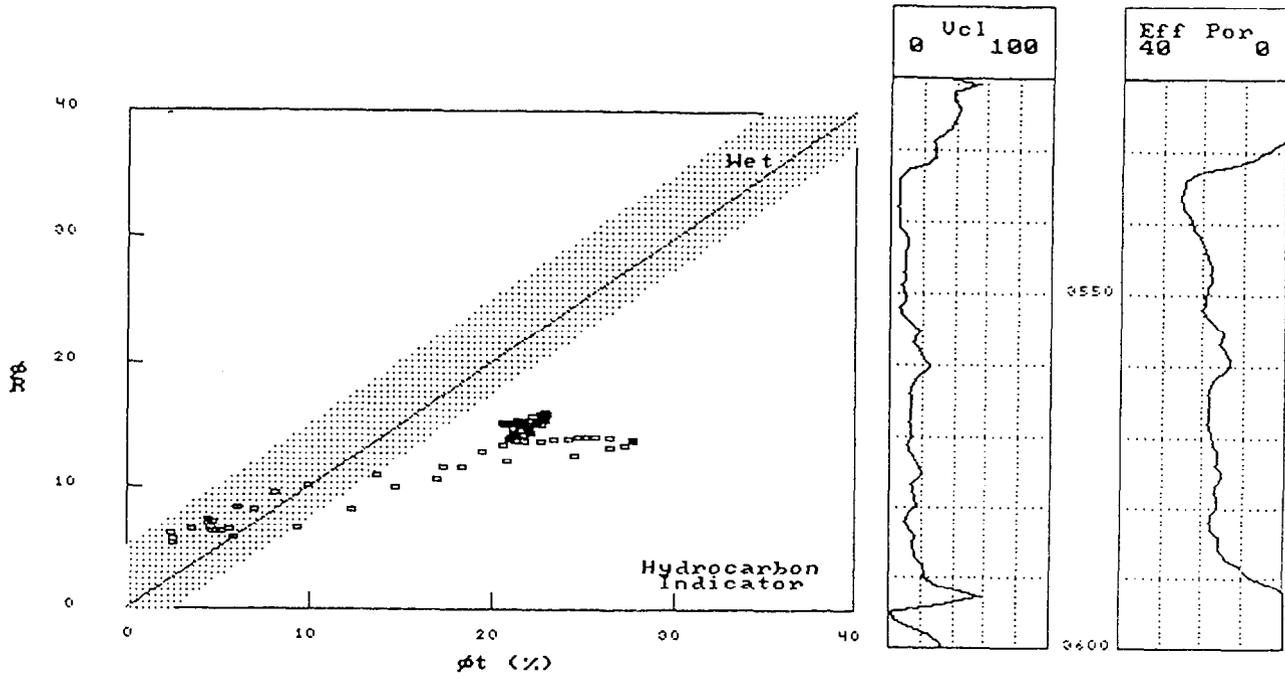
Figure 6 - Crossplot of invasion corrected deep resistivity ( $R_t$ ) Porosity ( $\phi_r$ ) versus total porosity ( $\phi_t$ ) for the Bell Canyon sand. The data that plot below the dotted pattern are from the porous sand from 1080 meters (3542 feet) to 1094 meters (3590 feet) and indicate the presence of hydrocarbons in the uninvaded zone. The zone should therefore be productive.
