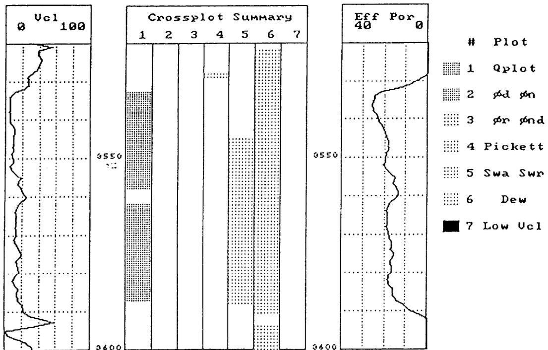
Figure 10b - Crossplot Summary for the potentially productive Bell Canyon sand from 1077 to 1094 meters (3532 to 3590 feet). Note that columns 3 and 4 (hydrocarbon versus water crossplots) indicate productive and column 5 indicates productive in the top 5 meters (16 feet). Only column 6 (Dew Plot) indicates water.
