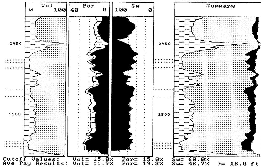
Figure 13a - Net Pay Summary for the potentially productive Bell Canyon (Ramsay) sand 741 to 770 meters (2430 to 2526 feet). Note that 5.5 meters (18 feet) of net pay is indicated with a concomitant hydrocarbon pore-meter thickness of 0.55 (1.8 pore-feet) using the following cutoffs:  $V_{cl} < 15\%$ ,  $\phi_e > 15\%$ , and  $S_w < 60\%$ .
