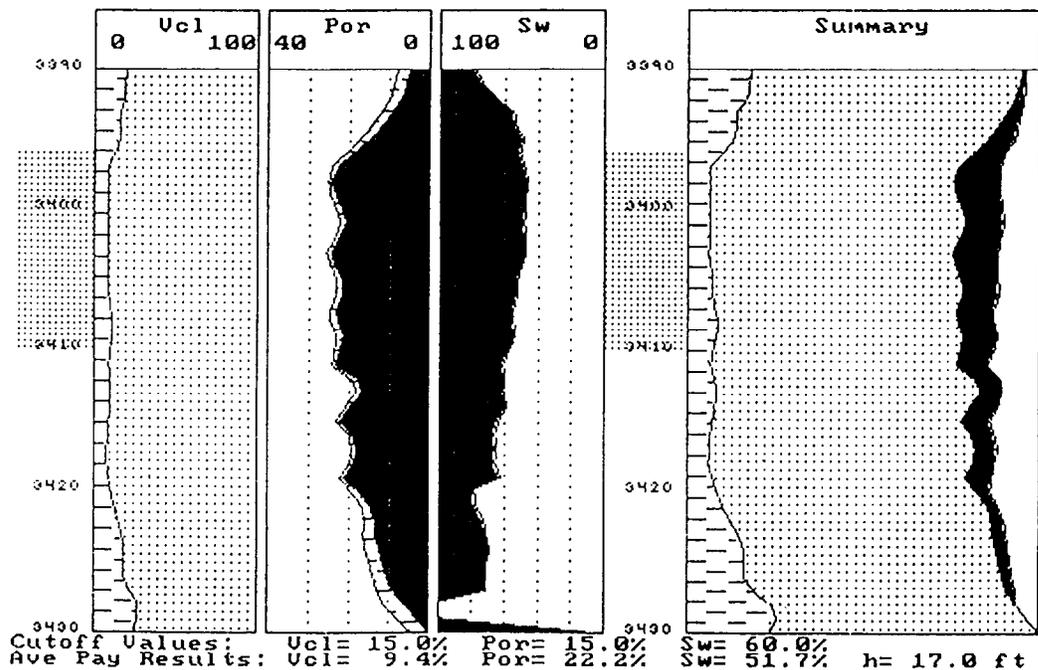
Figure 13b - Net Pay Summary for the potentially productive Cherry Canyon sand 1035 to 1044 meters (3396 to 3424 feet). Note that 5.1 meters (17 feet) of net pay is indicated with a concomitant hydrocarbon pore-meter thickness of 0.55 (1.8 pore-feet) using the following cutoffs:  $V_{cl} < 15\%$ ,  $\phi_e > 15\%$ , and  $S_w < 60\%$ .
