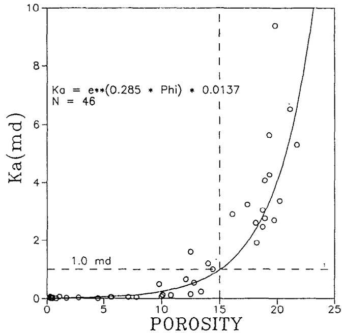
Figure 2 - Crossplot of core derived porosity versus permeability for the Bell Canyon and Cherry Canyon sands in Reeves and Culberson counties, Texas. Note that a porosity of 15% corresponds to a permeability of 1.0 md.
