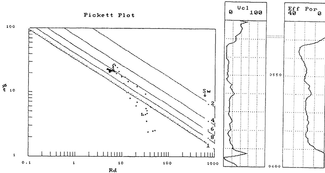
Figure 7 - Pickett Plot for the Bell Canyon sand. Note that a portion of the data plot above the  $S_w = 60\%$  line (i.e.  $S_w < 60\%$ ) and that none of the data plot on the  $R_o$  line (i.e.  $S_w = 100\%$ ). The data that plot well below the  $R_o$  line are the result of wash-out.
