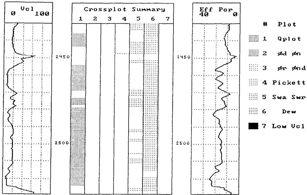
Figure 12a - Crossplot Summary for the potentially productive Bell Canyon (Ramsay) sand 741 to 770 meters (2430 to 2526 feet). Note that the permeable zones shown on column 1 are indicated to be productive on columns 3, 4 and most of column 5. Only column 6 (Dew Plot) indicates water.
