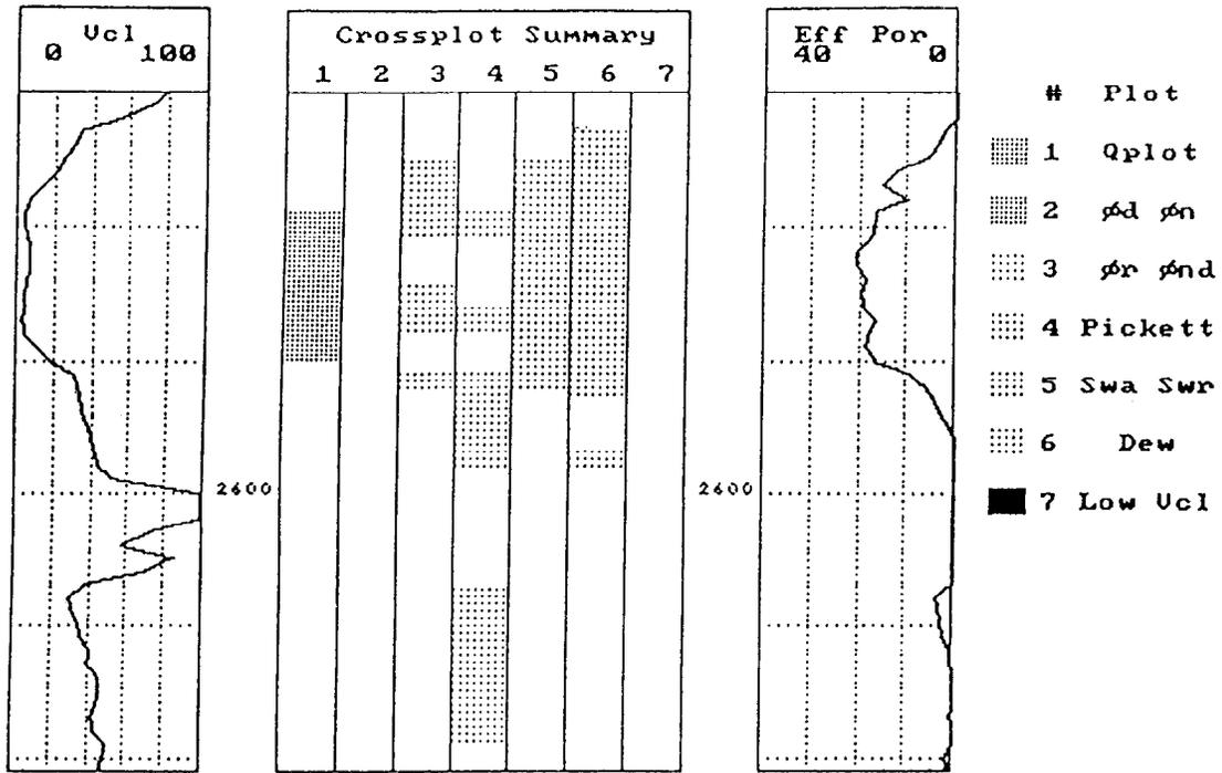
Figure 10a - Crossplot Summary for the water productive Bell Canyon (Ramsay) sand from 783 to 792 meters (2570 to 2600 feet). Note that on all the hydrocarbon versus water crossplots (columns 3 - 6), the Ramsay is indicated to be wet.
