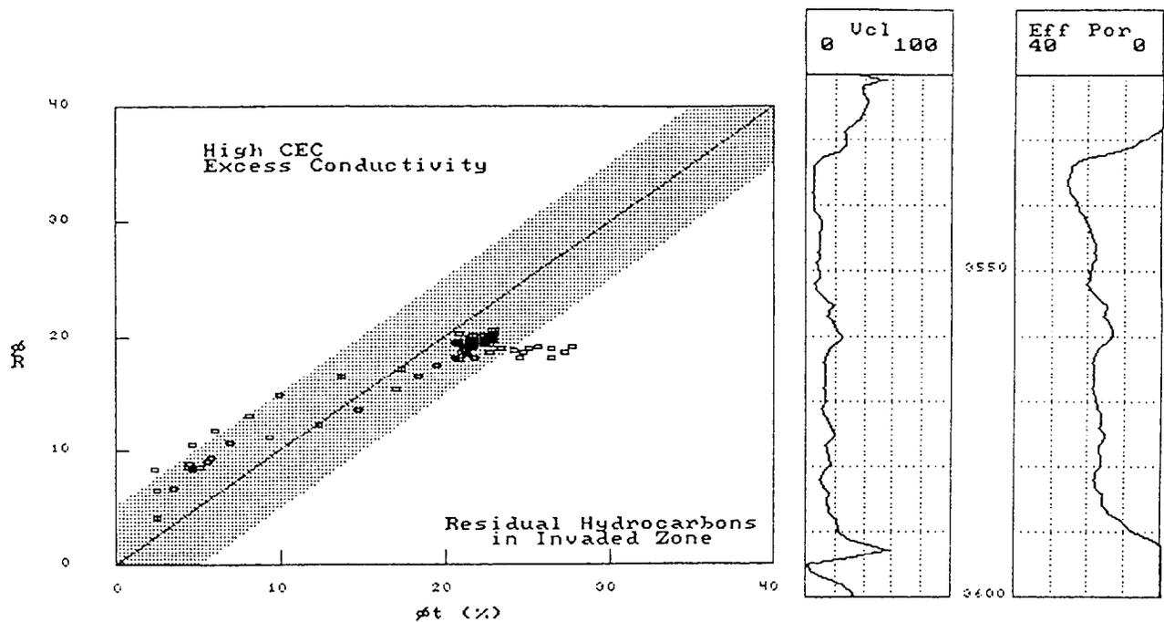
Figure 5 - Crossplot of shallow resistivity porosity ( $\phi_r$ ) versus total porosity ( $\phi_t$ ) for the Bell Canyon sand. The data that plot below the 45 degree line ( $\phi_r = \phi_t$ ;  $S_w = 100\%$ ) represent residual oil in the invaded zone. The data that plot below and outside the dotted pattern represent the higher amounts of residual oil present in the top 6.1 meters (20 feet) of the zone.
