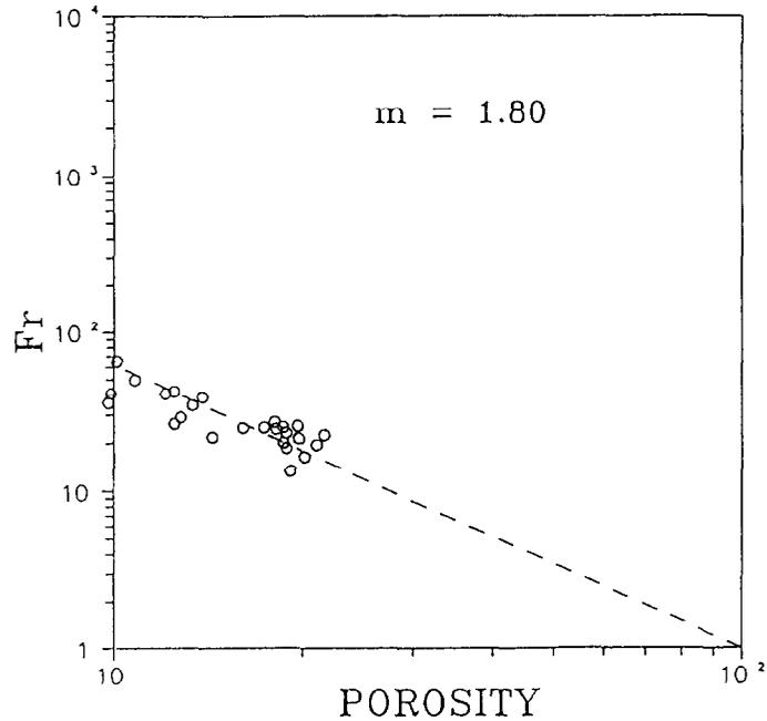
Figure 3 - Crossplot of formation resistivity factor (Fr) versus core porosity for the Bell Canyon and Cherry Canyon sands in Reeves and Culberson counties, Texas. The slope of the best fit line (slope = 1.80) represents the average cementation exponent (m) for the Bell Canyon and Cherry Canyon sands.
