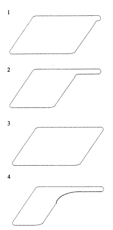
This is the ideal downhole card if the fluid level is at the pump or slightly over the pump.
