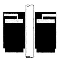
A pump indicator is a hollow bore hydraulic cylinder located between the carrier bar and the rod clamp. It indicates the amount of load carried by the Carrier bar.
