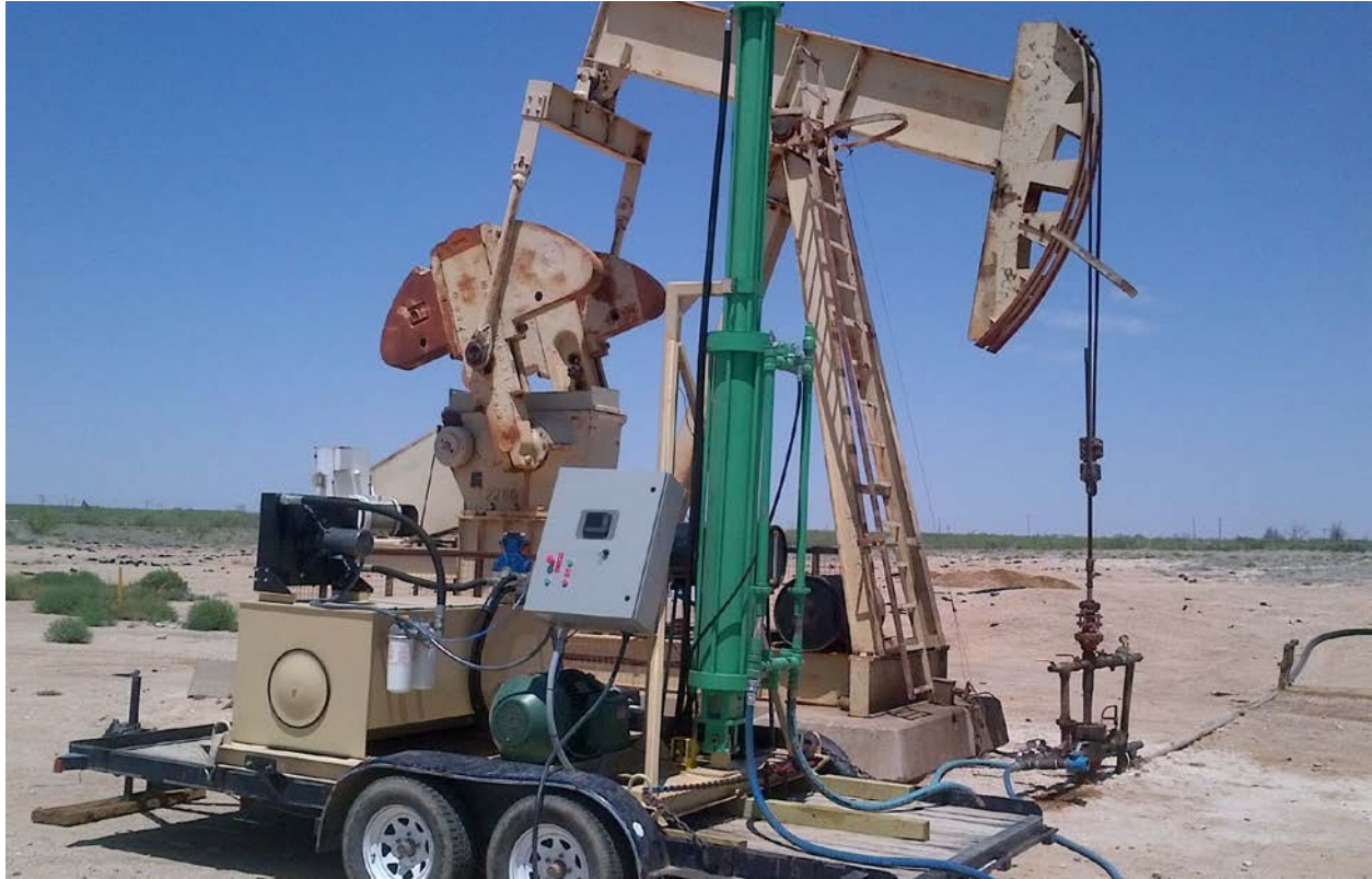
HyBGC on location as a wellhead compressor
