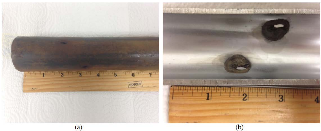
Figure 4 - Helical honing marks on the barrel surface.
