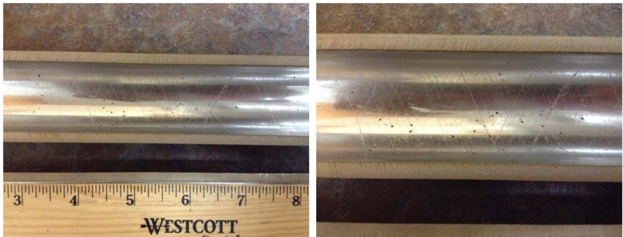
Figure 4 - Helical honing marks on the barrel surface.
