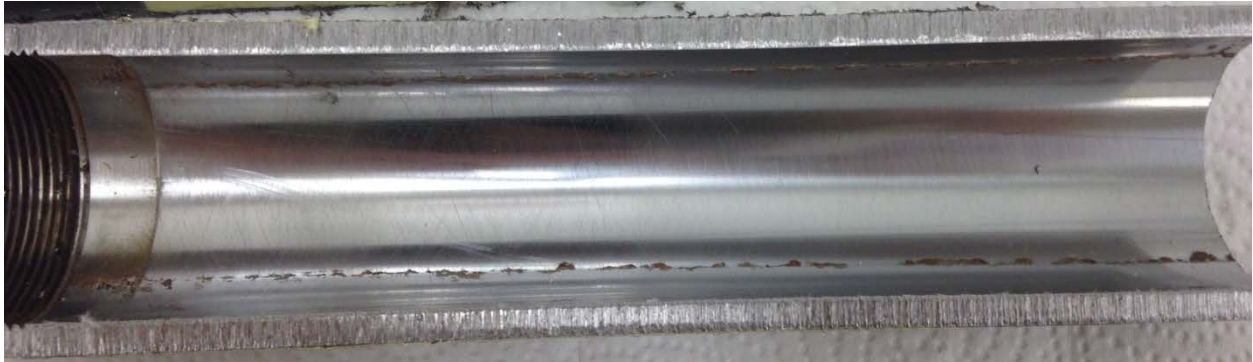
Figure 7 - Pits aligned on a straight line on the barrel surface.
