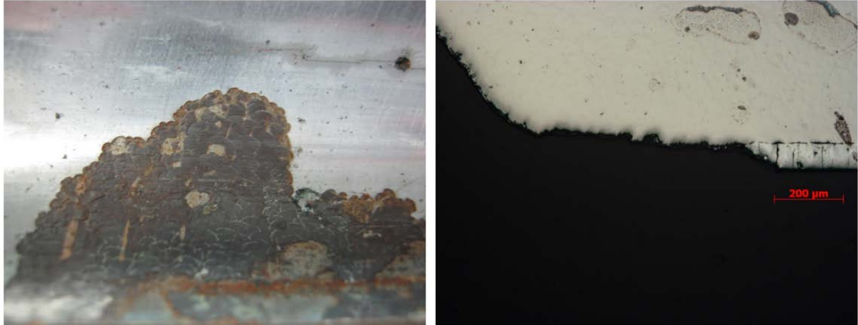
Figure 6 - Flaked Chrome coating on the barrel surface.
