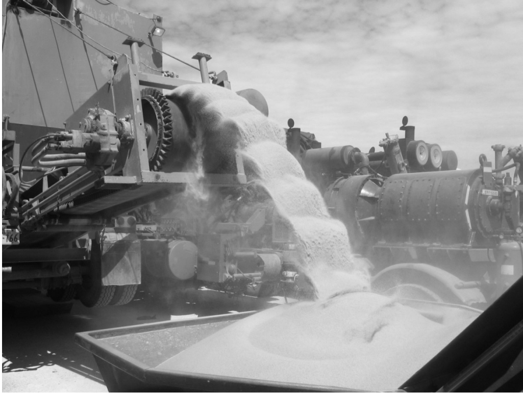
Figure 1 – Proppant sampling point from conveyor to blender hopper
