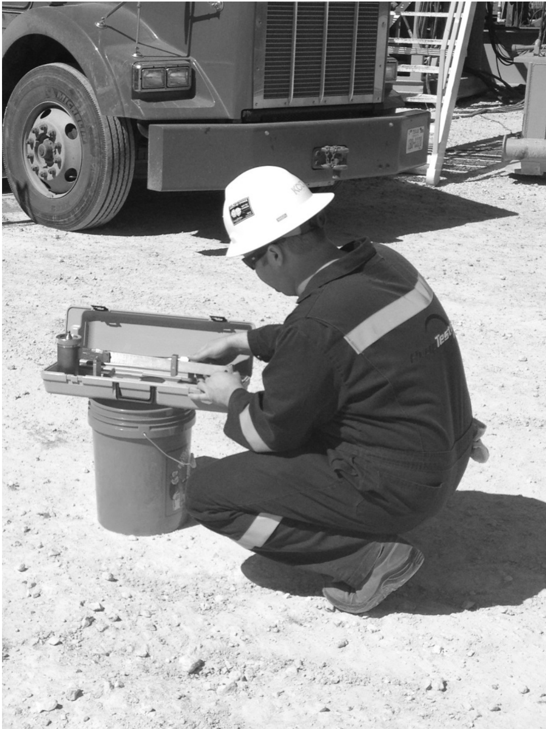
Figure 1 – Use of Pressurized Mud Scale
