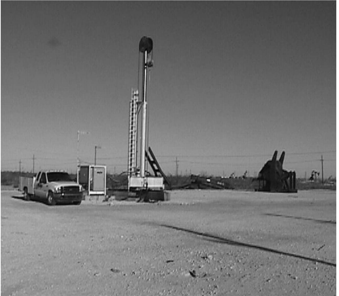
Figure 4 - A Model 9 DynaPump Replaces a Lufkin 912 on Well # SWCU 8545
